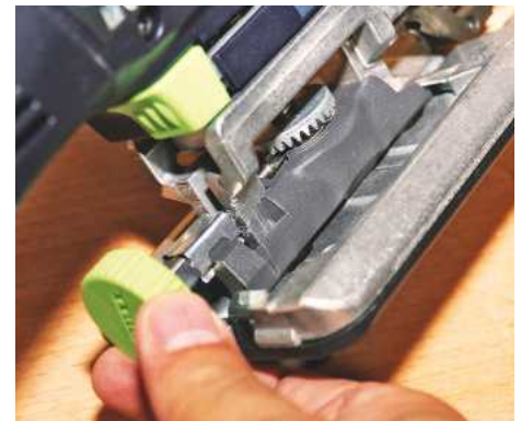
▲ Any bevel cuts are made with adjustments to this clever piece of kit
